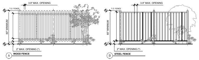
(\*) NOTE FOR WOOD & STEEL FENCE: 4" MAX. OPENING ALLOWED WHERE SURFACE BELOW IS CONCRETE OR ASPHALT.
